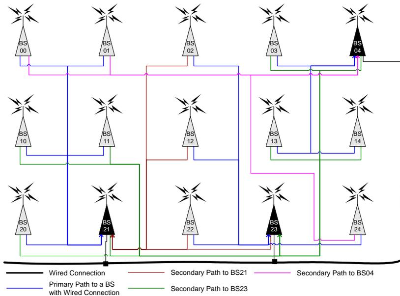
**Figure 1: Typical Primary and Secondary Mesh Connectivity**
