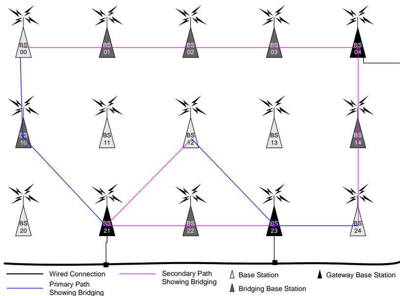
**Figure 2: Base Station Capabilities for a Network Subset**
