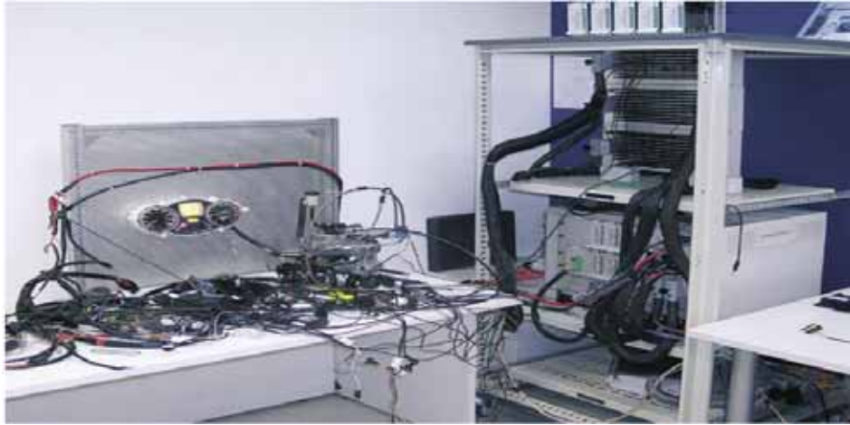
Figure 3-12 The hardware-in-the-loop setup with a dSPACE Simulator Mid-Size
