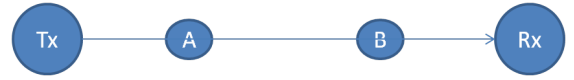
Fig. 4. Single-path (SP) topology. The message originates from Tx, and is passed along the relay nodes (A and B), before finally arriving at the destination node Rx.
