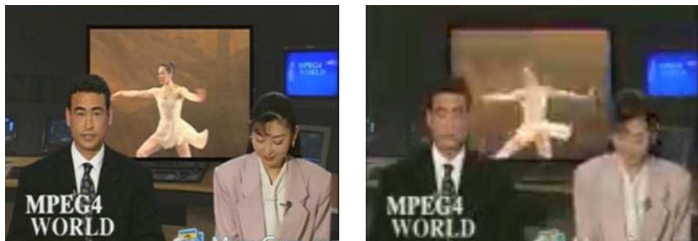
Figure 4.5: Original and degraded video frames transmitted at 5% packet loss from application using Skype resulting in PSNR=24.49
