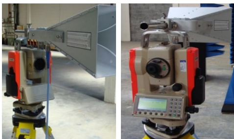
Fig. 3: Antennas mounted on a modified Pentax Precision Total Station
