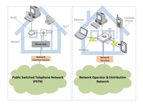
Figure 2.1: Wired and Wireless Connections Home Area Network - Showing the limitations of Wired Network from mobility point of view
