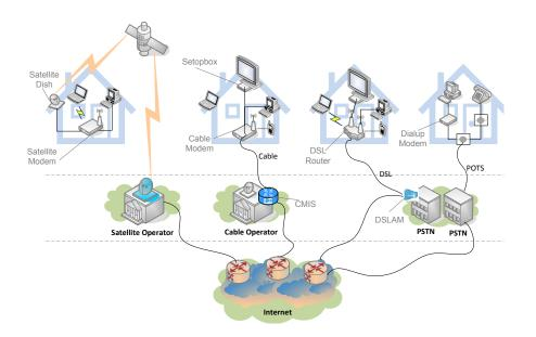
Figure 2.2: POTS, DSL, Cable and Satellite ISP connections for Home Area Networks.
