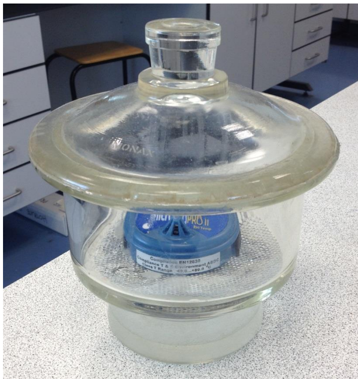
Figure 3.10: Image of sealed humidity chamber set-up with saturated sodium bromide solution and data logger.
