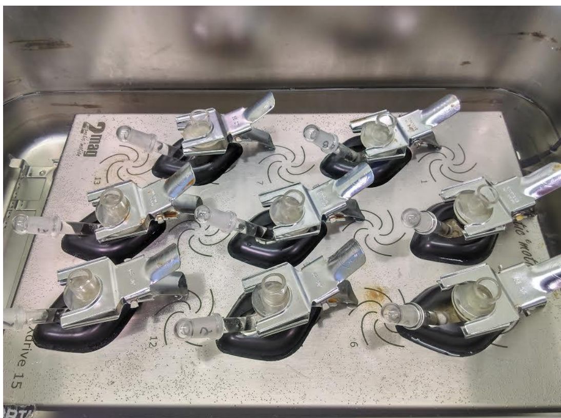
Figure 4.10: Franz diffusion cells set up on a Mixdrive 15 multi-position magnetic stirrer in heated water bath.
