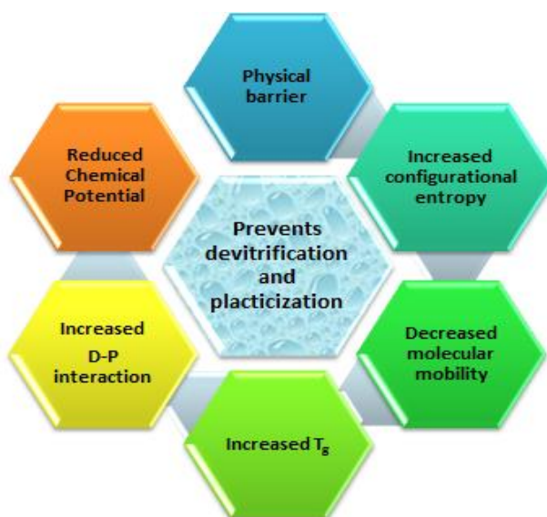
Figure 1.5. Different approaches for stabilizing the amorphous solid dispersion in a polymer matrix; D-P represents drug-polymer and T g represents glass transition temperature.
