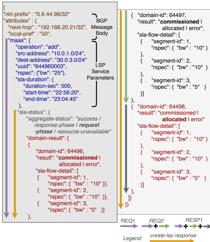
Fig. 3.11 Different MaaS-Fed messages illustrated in their JSON format in relation to the considered example scenario.
