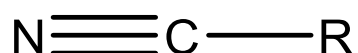
Figure 1.1 General structure of nitrile compounds with the triple bonds observed between the carbon and nitrogen
