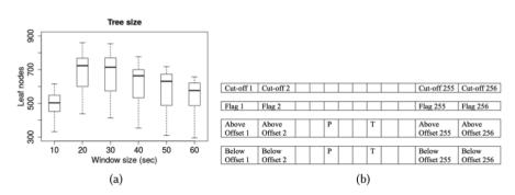
Fig. 25. (a) Effect of windowSize on the size of DT (b) Array-based implementation of DT.
