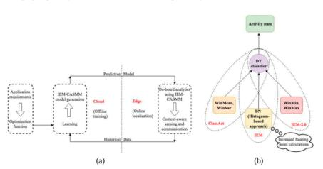
Fig. 1. (a) System architecture (b) ClassAct-, IEM-, and IEM-2.0-based classification.
