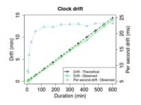
Fig. 11. Clock drift incurred by a collar device over time.
