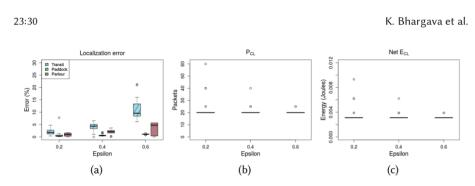
Fig. 24. Effect of ASMM on (a) Localization error (b)  $P_{CL}$  (c) Net  $E_{Cl}$  for windowSize = 60 and N' = 5.
