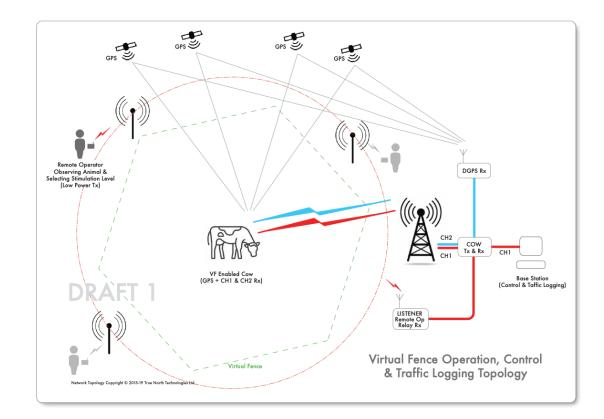
Figure 5.1: Topology design for the communion infrastructure of the virtual fence VF system. The communication methodology linking the operator, base station and the VF collar on the cow using channel 1. Channel 2 describes the implementation of the DGPS correction via the DGPS receiver system and the VF collar on the cow.
