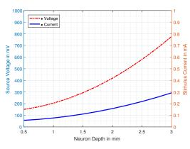
Fig. 8: Plot of stimulus current and source voltage for a range of neuron distances and a chronaxie of  $100\mu$ s. The further the neuron is from the nanodevice array electrode the higher will be the required stimulus voltage/current.
