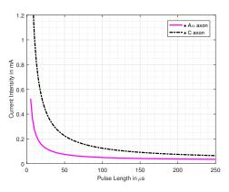
Fig. 7: Plot of current against pulse duration for two types of axon, one myelinated (A $\alpha$  axon) and one unmyelinated (C axon). The current intensity for a pulse duration of 100 $\mu$ s is less than 0.2 mA.
