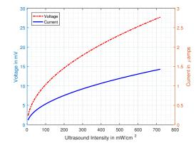
Fig. 6: Plot of ultrasound intensity against output voltage and output current for a  $1000\mu m^2$  nanodevice at an ultrasound frequency of 50kHz.
