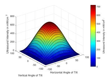
Fig. 5: Plot of Ultrasound Intensity vs Angles of Tilt for a frequency of 50kHz and a skin/fat depth of 5 mm. The tilting of the nanodevice will have a significant impact on the incident ultrasound intensity.
