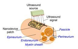
Fig. 1: Bio-compatible patch containing nanodevice array powered by externally generated ultrasonic waves. The array sends current pulses to stimulate specific *fascicles* (nerve fibre bundles).
