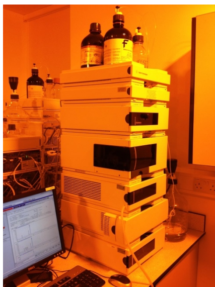
Figure 3.6. Agilent Technologies 1200 high-performance liquid chromatography (HPLC) system used for carotenoid analysis, operated under amber light.
